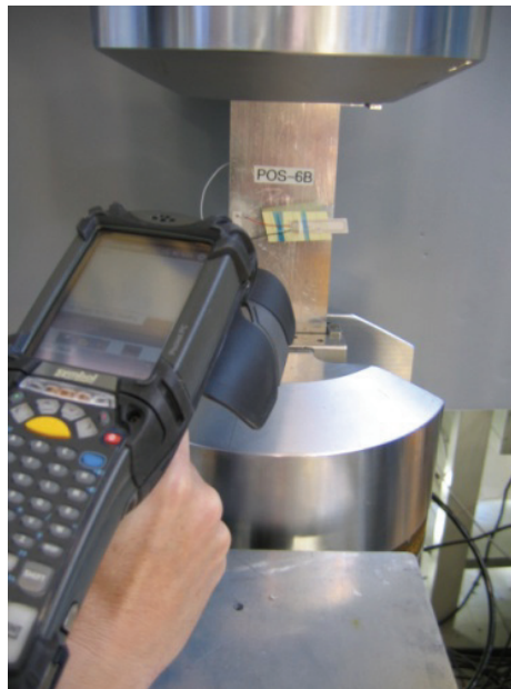
Fig. 20. Illustration of an RFID-based crack detection approach.
